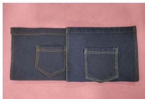
Figure 3. Neutral bio-polishing on Denim jeans with ECOENZYME - TXT NCL BP
