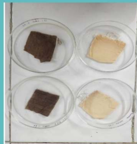
Figure 1. ECOENZYME - TXT LTAL CONC Tegawa results (Iodine test) on Cotton and Viscose rayon.
